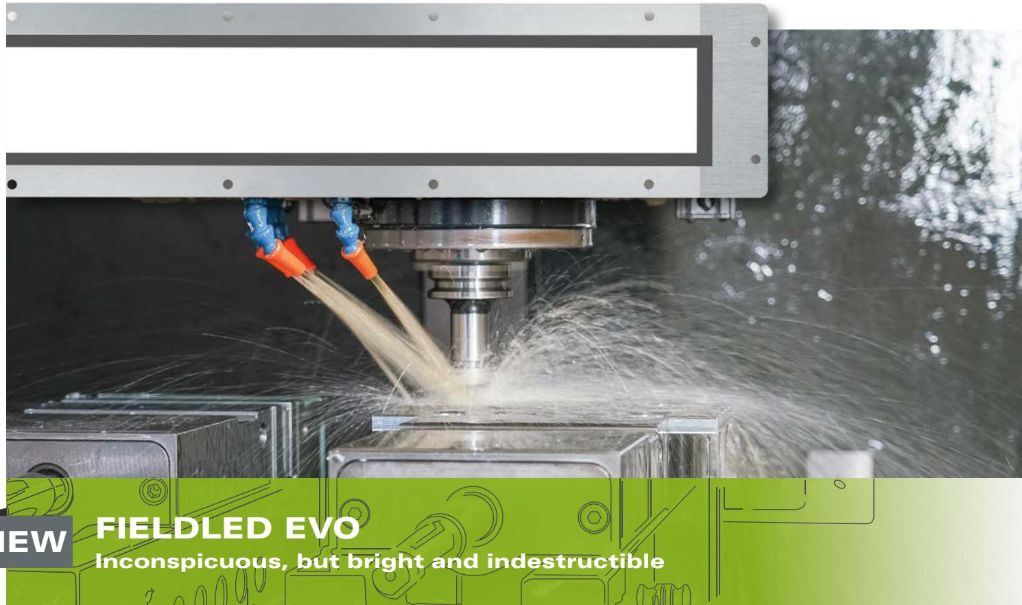
The recessed FIELDLED EVO is the perfect machine light thanks to its precise-fit installation and powerful illumination. It was developed for harsh production environments and remains completely untroubled by chips, oil and emulsions. The safety glass is glued to the aluminium housing. An additional oil-resistant seal encloses the installation frame against the machine housing. Even in its recessed variant, the FIELDLED EVO comes with the highest protection rating and is utterly indestructible.
